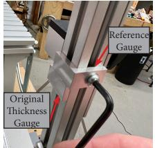
Once the Thickness Gauge XL is in the desired location, slide the original Thickness Gauge up to contact the bottom of the XL and slide the reference gauge down to contact the original Thickness Gauge. In the unlikely event that the Thickness gauge needs to move for an operation, slide both original and XL Thickness Gauges down out of the way and leave the reference gauge in place to have a positive stop to return to.
