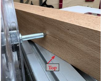
Flip the workpiece 180 degrees so the face marked "Top" is now against the table. If the Thickness Gauge XL is in the correct location the pointer should line up with the scribed mark.
