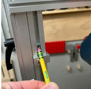
Slide a pencil under the nut and remove the hex wrench.
