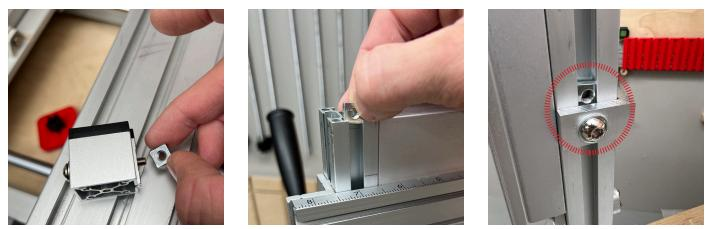
Remove the square T-slot nut from the back of the new Thickness Gauge XL and drop it in the front T-slot of the Template Holder Support Frame. It will land on top of the original Thickness gauge.
