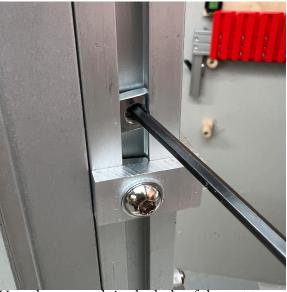
Use a hex wrench in the hole of the nut to lift the nut up from the existing Thickness Gauge.
