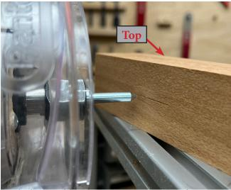
With the Double-Point Centering Jig in the router and the face marked "Top" facing up, move the wood across the pointer to scribe the centerline on the sample workpiece.
