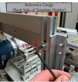
Using a 4mm hex wrench, loosen the screw for the thickness gauge and slide it down towards the table. Next, slide the reference gauge on the back side of the Template holder support frame up and out of the way.
