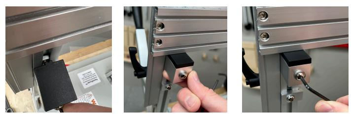
Align the screw of the Thickness Gauge XL with the nut and loosely thread it in. Slide the Thickness Gauge XL up until it contacts the bottom of the Template holder and Tighten it in place using a 3mm hex wrench.
