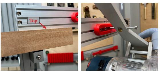
lever knobs and insert the 6mm shaft of a guide bearing in the center hole of the Template Holder. Mark the face contacting the bottom of the Template Holder with the word "Top".
