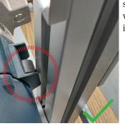
some locations, however, there should be no position in which the router switch itself can be moved by contacting the machine.
