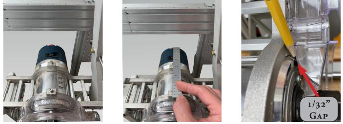
When installing the router in the Router Mounts make sure the router controls are in line with the Router Locking Screws before tightening. A small ruler resting on top of the two Router Locking Screws can help with proper alignment. The router should be pushed forward in the Router Mounts so the bevel of the router motor clears the front router mount and is held back from the dust hood about 1/32" (0.8mm).
